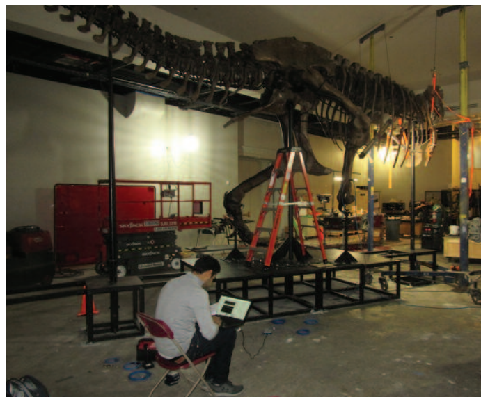
Figure 2. Vibration testing underway in the new SUE gallery during gallery construction.
