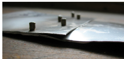
Solder not fully sweated through this twenty-two-gauge stainless steel lapped, riveted, and soldered seam. The rivets are too long as well.
