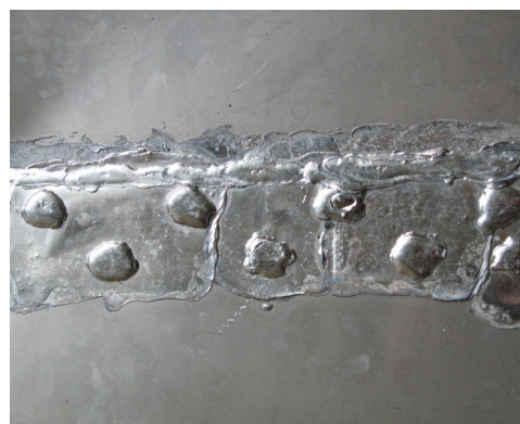
Solder not fully sweated through this twenty-two-gauge stainless steel lapped, riveted, and soldered seam. The rivets are too long as well.
