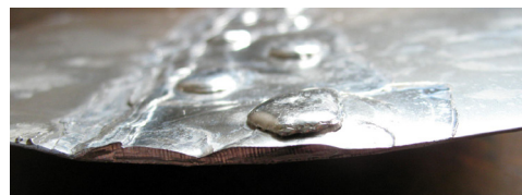
Top surface (top) and cross section (bottom) of a twenty-two-gauge stainless steel lapped, riveted, and soldered seam with solder fully sweated all the way through. Soldering was performed using the methods described on the reverse.
