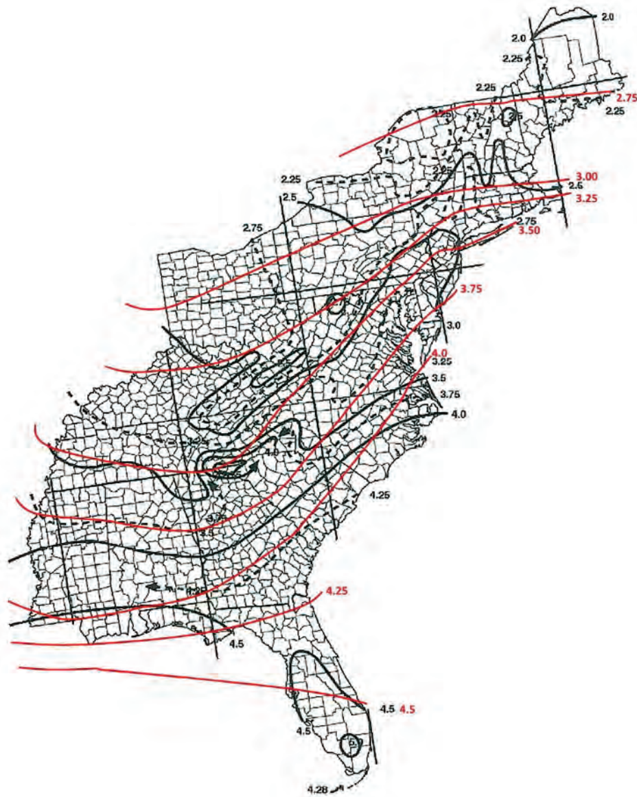
Figure 6. Yarnell’s 100-year, 60-minute isohyets 6 (shown in red; locations are approximate) overlaid on the 2021 International Plumbing Code 3 Figure 1106.1, “100-Year, 1-Hour Rainfall Map of the Eastern United States.” The isohyets have become more convoluted and generally shifted to the south over time.
