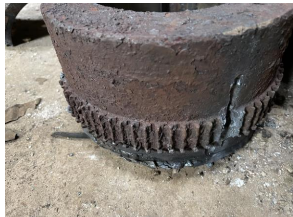
Figures 8 & 9: Photos showing the internal condition of the failed coupling. Note excessive wear and corrosion on gear teeth, with similarity to couplings shown in Case I. Also shown burn marks were inflicted during coupling disassembly from shaft.
